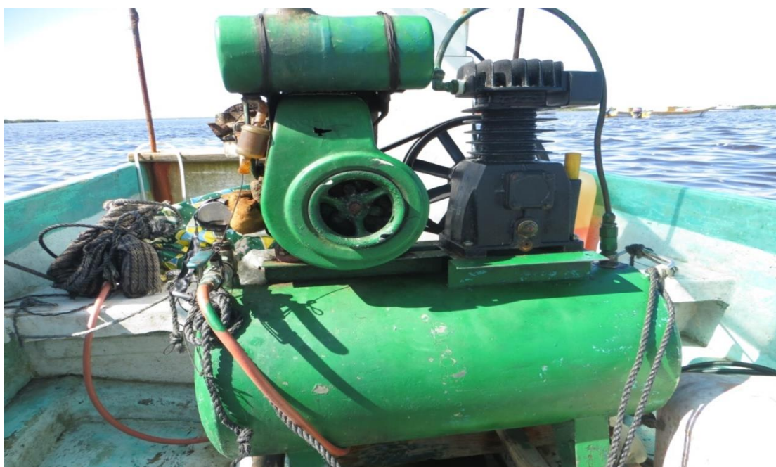
Figure 1. The diving hookah system
